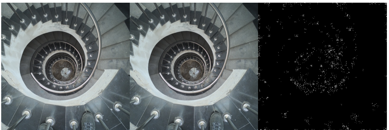
Figure 5.2: Clean image, image with UERD embedded data, scaled differential image between them. The average embedding rate is 0.4 bpnzAC.
