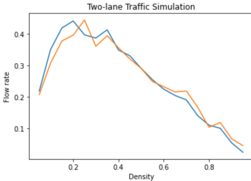
Figure 4.8: Average flow rate for 15 time steps for two lanes. For the two-lane model, the max flow rate is: 0.44000000000000001 and it's reached at the density of: 0.06
