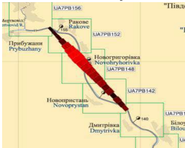
Fig. 3. Change of the speed of the river flow by changing the angle of slope of the middle bottom line.
